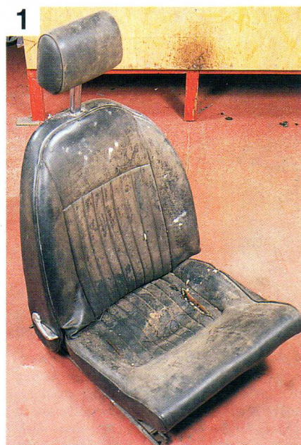
This is what we started with – a typical well-used Spitfire seat with a split in the tired vinyl cover. Our seats (Spitfire Mk IV, 1500 and GT6 Mk 3 are all the same) were obtained from AD Autos
