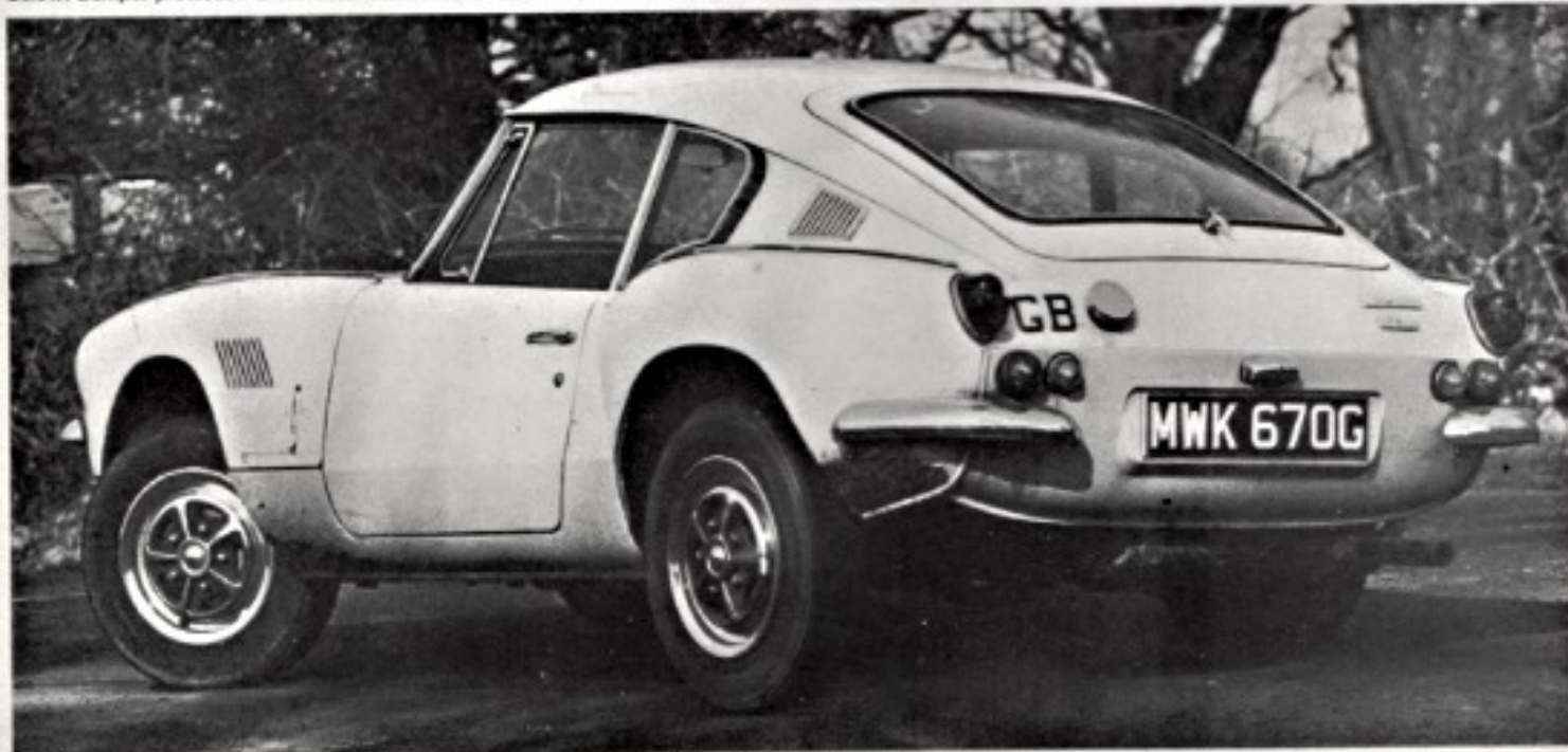
Below: Bumper protection at the back is minimal, and the lamp clusters are in need of tidying up. Fancy wheels are dummies in the form of stainless steel trims
