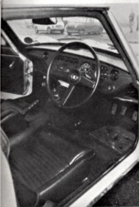
Top right: Wheel camber is well controlled now, thanks to rear-end revisions. The bars on the window are for the heated glass. Above: Non-gloss wood veneer, a padded wheel and new switches are features of the Mk. 2 GT6. Fresh-air vents are new too
